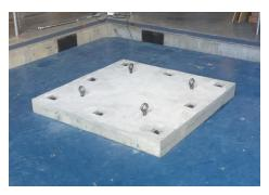
Figure 2. Concrete slab installed on the Shake Table.
