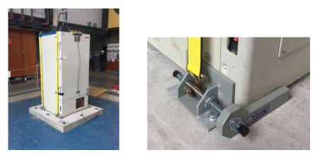
Figure 3. Test setup and EQ Restraint System (EQRT 203-7) installed on the equipment prior to testing.
